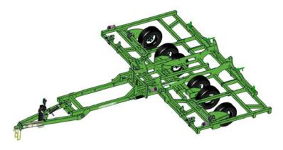
CropCadet™ is the ultimate direct drill seeding machine is designed to meet the needs of farmers seeking flexibility and durability. Perfectly suited for 200-250 HP tractors, it offers a high underframe for better residue and trash flow through the machine, ensuring optimal performance.
